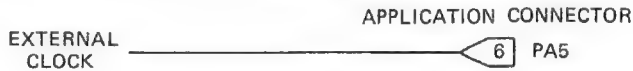
FIGURE D-2. Connection of the external clock to bit 5 of port A of the user 6530 device. (Note: Jumper wires can be used to select either this input or the switch input shown in Figure 2-1.)
