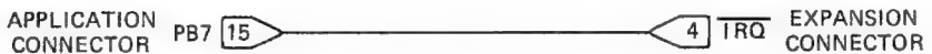
FIGURE D-3. Connection of pin PB7 of the user 6530 device (the timer interrupt request) to the microprocessor's \overline{\text{IRQ}} input. (Note: Jumper wires can be used to select either this input or the LED output shown in Figure 3-1.)
