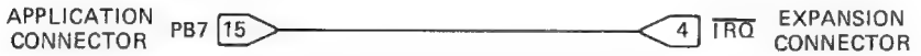
FIGURE A4-13. Connection of pin PB7 of the user 6530 device (the timer interrupt request) to the microprocessor's IRQ input. Note: Jumper wires can be used to select either this output or the LED output shown in Figure A4-2.
