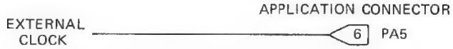
FIGURE A4-12. Connection of the external clock to bit 5 of user 6530 port A (address 1700 hexadecimal). Note: Jumper wires can be used to select either this input or the switch input shown in Figure A4-1.
